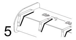
Apply small amount of CA glue on the edge of the 3 center support ribs and allow it to dry.
