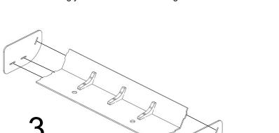
Line up the slot on the spoiler end plate with the tabs on flaps then insert and connect them together
