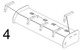
Place and glue (CA glue) the side support ribs (2 pieces) on bottom side of the flaps (making sure the support ribs are contacting the end plate)
