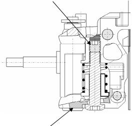
When bottom of A-Arm is horizontal with ground, suspension is at stock ride height. Each additional <sup>1</sup>/<sub>4</sub> turn of spring guide screw drops ride height by .2mm, or 1 washer equivalent of suspension drop.
