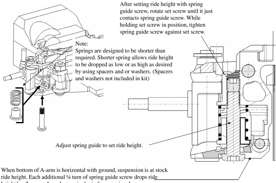
height by .2mm, or 1 washer equivalent of suspension drop.
