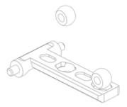
Insert both Delrin Balls vertically as pictured into the oval slot
