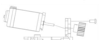
Insert narrow portion of the pinion gear through motor mount,
