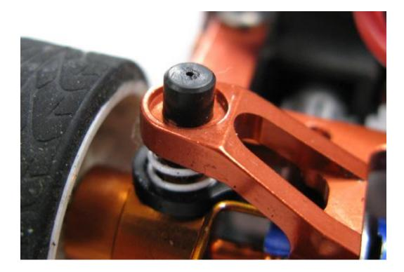
Install Damping Cap onto upper cover and install rest of suspension components.
