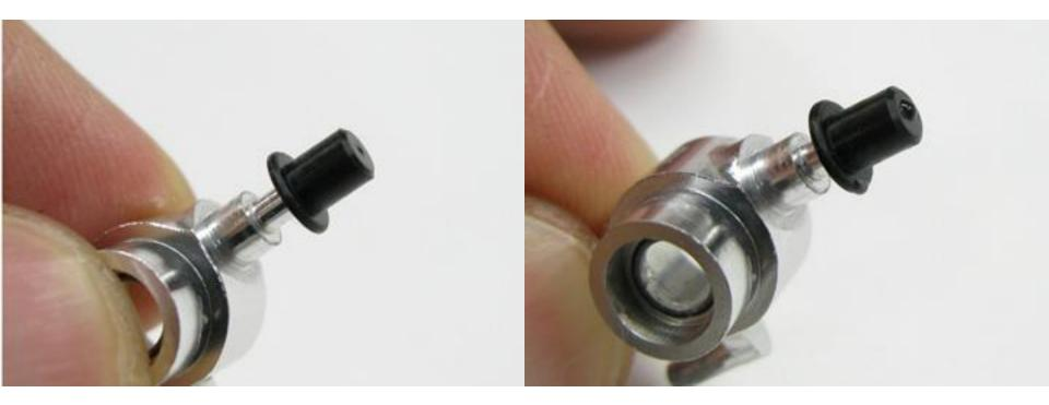
Insert damping cap onto top post of the knuckle. Cycle cap on knuckle suspension post to distribute damping fluid. Wipe off excess fluid from the vent hole.
