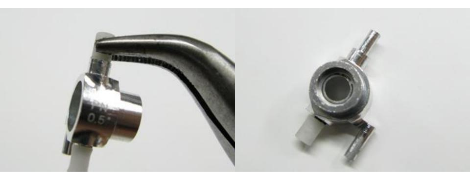
Remove knuckle delrin collar using pliers. Be careful not to scratch the suspension post on the knuckle. Remove only upper collar, do not remove lower collar.
