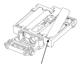
1. Insert battery into front of the chassis first
