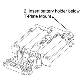
3. Push down battery clip to latch on chassis
